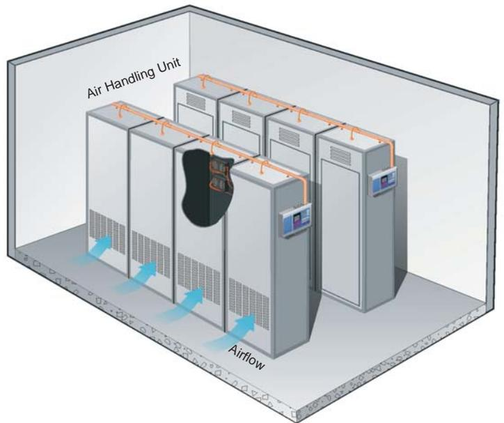
Fig 4. In-Cabinet Capillary Sampling for Switch Rooms
