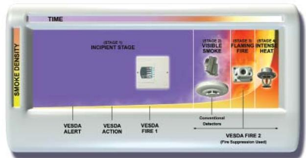
A VESDA smoke detector can be configured to detect a fire at the earliest stage. The multiple alarm levels can be configured to initiate an appropriate response at all stages of a fire.
